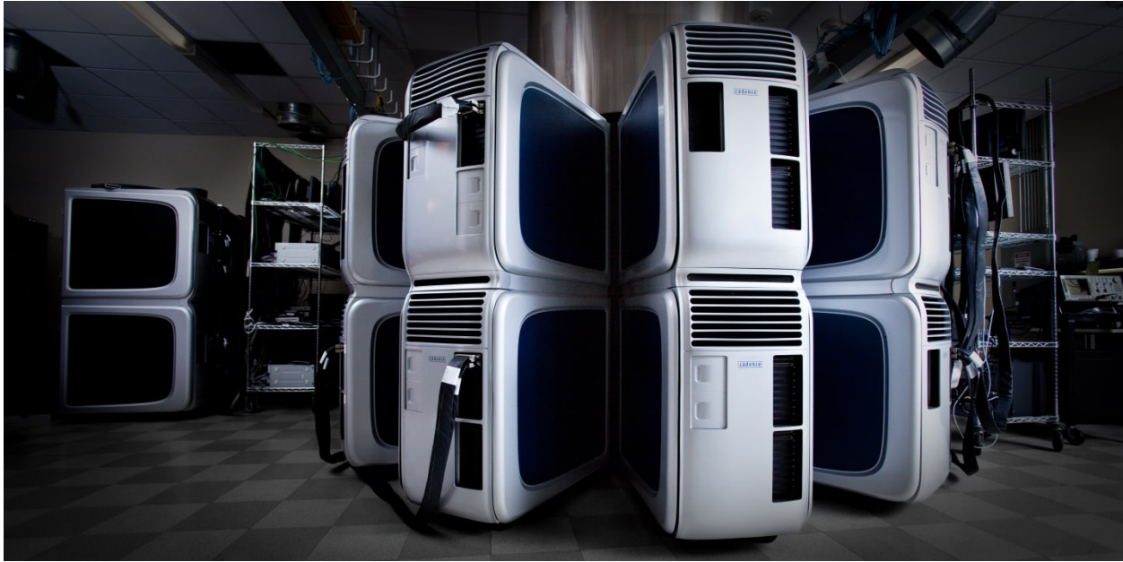
Fig. 9: An entire room-scale Cadence Tigris emulator 9
